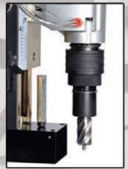
Kernbohren core drilling
