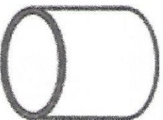
#17 Receiving tube O.D.: 2-1/2" I.O.: 2-1/4" Length: 2-3/4"
