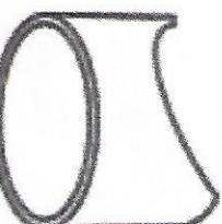
#15 Receiving tube O.D.: 3" I.O.: 2-3/4" Length: 2-1/4"
