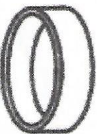
#07 Receiving tube O.D.: 2-1/2" I.O.: 2-1/4" Length: 3/4"
